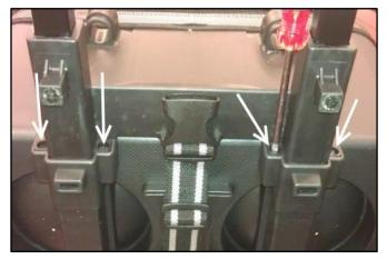
**Step 9**. Slide the bottom bag rack into place. NOTE: It will take some taps with the hammer and alignment to get it fully into place, and the holes for the screws must line up with the holes on the rack.
