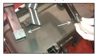
**Step 6.** Make sure the replacement handle is fully collapsed and that the outer sleeves are pushed all the way up into the handle. NOTE: it will take some adjusting to get the sleeves to fit into the square openings.
