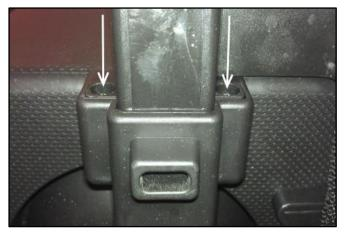
**Step 8**. Replace the (4) screws from step 3. NOTE: If the screws are all the way in but keep spinning or don't get tighter, this is ok and can be left alone.
