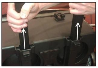
**Step 5.** Save the intermediate wrapped sleeves that are on the bottom rails. These are very important and MUST be on the replacement handle in order for both locking stages to work.
