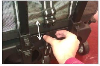
**Step 2.** Remove the bottom bag rack screws, (5) total. Slide the rack away from handle.
